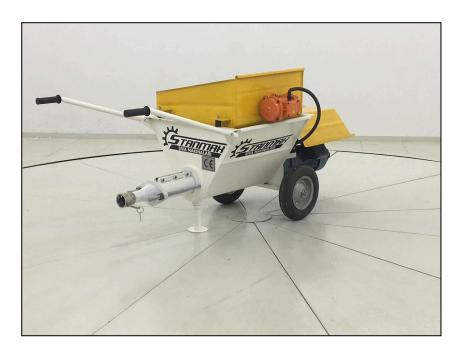
Material Used: Sand, Cement, Lime Pumping Capacity: 75 – 1/min Pumping Pressure: 20 bar Pumping Distance: 15 –25 m
