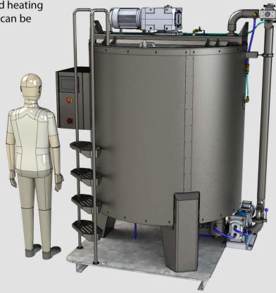
Chocolate storage tank we produce is cylindrical. It is water jacketed with PID controlled heating element. Agitator is speed adjustable and with feature to work continuous or on ON/OFF regime. Water inside a twin-shell coat ensures heating and keeping temperature of chocolate mass constant. Chocolate storage tank is used to store the liquid chocolate in constant temperature and homogenous structure. They are not suitable for melting purposes.
