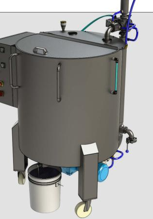
Chocolate storage tank we produce is cylindrical. It is water jacketed with PID controlled heating element. Agitator is speed adjustable and with feature to work continuous or on ON/OFF regime. Water inside a twin-shell coat ensures heating and keeping temperature of chocolate mass constant. Chocolate storage tank is used to store the liquid chocolate in constant temperature and homogenous structure. They are not suitable for melting purposes.
