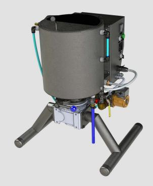
LabBM10 is designed for laboratory use, product development or educational use. Machine is equipped with solenoid valve which automatically opens gate of cold water flow and ensures cooling of the equipment. Because of friction of spheric balls cold water is required from an external source which can be from tape, tower or a chiller. Machine will open cold water gate in case overheating and will close it when cooled.
