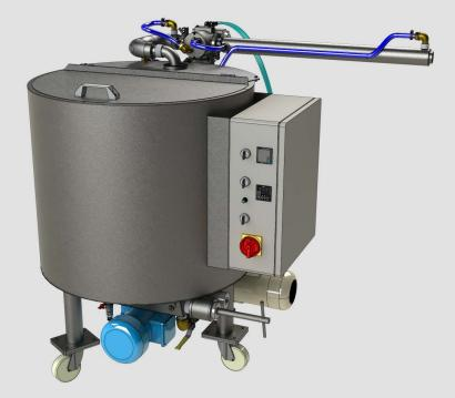
Chocolate storage tank we produce is cylindrical. It is water jacketed with PID controlled heating element. Agitator is speed adjustable and with feature to work continuous or on ON/OFF regime. Water inside a twin-shell coat ensures heating and keeping temperature of chocolate mass constant. Chocolate storage tank is used to store the liquid chocolate in constant temperature and homogenous structure. They are not suitable for melting purposes.
