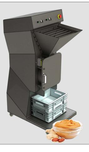
Cocoa nib grinder is made of stainless steel and designed for small workshops. Grinder is able to grind roasted hazelnuts, peanuts and cocoa beans up to 500 microns. While the upper part of the grinder cracks roasted nuts, having pins bottom part of the machine turns the roasted nuts into a thick paste. The paste then can be thinned in ball mills up to 18 microns. Pre-grind roasted whole nuts into thick paste up to 500 microns.
