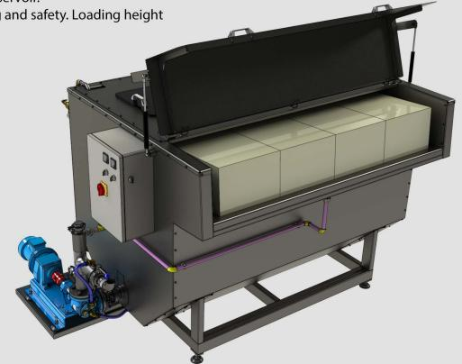
Fat melting tank we produce is rectangular in order to provide maximum melting area. They are with glass wool insulation and PID controlled heating element. Other importent thing we pay attention on our designs of melting machines is the loading height. Loading of solid blocks should be with minimum effort. We mount grid with separate hot water circulation to achive faster melting process.
