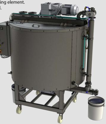
Chocolate melting tank we produce is cylindrical. It is water jacketed with PID controlled heating element. Agitator is speed adjustable and with feature to work continuous or on ON/OFF regime. Water inside a twin-shell coat ensures heating and keeping temperature of chocolate mass constant. Chocolate melting tank is used to melt solid chocolate and store the liquid chocolate in constant temperature and homogenous structure.
