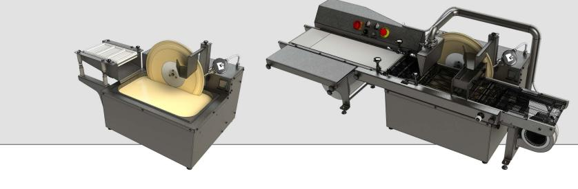
TTWBTM20 is table top wheel tempering machine ideal for beginners or patisseries. Tempering operation is made manually by adding some solid chocolate drops to melted chocolate. Machine is equipped wth 2 cooling fans for faster cooling. Vibration table, enrobing belt with bottom coating and full coating can be coupled.
