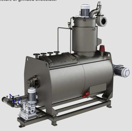
Low energy consumption fluid conche with single shaft agitation equipped with specially designed mixing arms. Vertical heated reservoir for chocolate splashing and air suction for removing the acidity and moisture.
