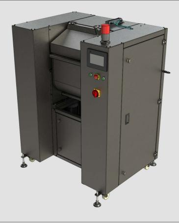
Z kneaders are horizontal type mixing devices. Rotation forward up to 110 degrees is performed by hydraulic tilting mechanism. Single arm z kneaders are suitable for hard biscuit dough, cookies, crackers, tortillas, stiff fillings and pet foods. Double arm z kneaders are suitable for many applications such as mixing and kneading different kind of dough like soft biscuit dough, cake dough, different creams and fillings.
