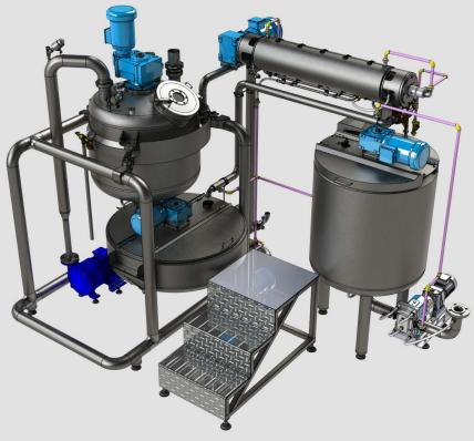
The main component of the caramel manufacturing plant is caramel cooker. Cooker is hemispheric and it is with Teflon scrapers. Agitation speed of the cooker is adjustable. Caramel cooking plant is equipped with HMI and PLC. Water jacketed takeoff reservoir with agitation, heat exchanger with helix rotor, fondant beater, vacuum pump and storage tank are other components of the plant. Fondant beater is required for the fondant manufacturing process.
