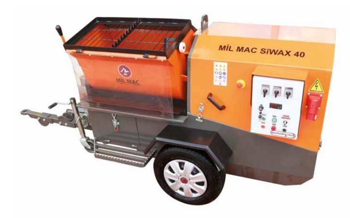
MILMAC SIWAX 40 Mortar plaster, double drum tumbler, tilting drums allow quick and homogeneus mixture. Auto lubricating pump increases the durability of reductor gears.
