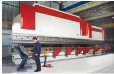
Abkant Pres Tandem Asimetrik 8100/4100 mm x 800/440 ton Press Brake Tandem Asymmetric 8100/4100 mm x 800/440 tons
