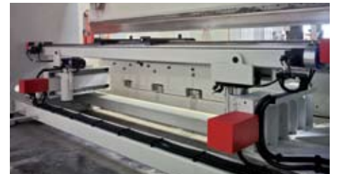
Ağır tip altı eksen arka dayama (X1-X2-R1-R2-Z1-Z2) Heavy duty six axis backgauge (X1-X2-R1-R2-Z1-Z2)
