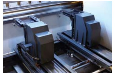
Konsol tip arka dayama (X1-X2-R1-R2-Z1-Z2) Tower type backgauge (X1-X2-R1-R2-Z1-Z2)
