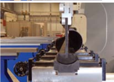
Abkant Pres Tandem Asimetrik 8100/4100 mm x 800/440 ton Press Brake Tandem Asymmetric 8100/4100 mm x 800/440 tons
