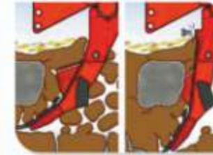
Yük Halinde Makineyi Koruyan Pin Emniyetli Bacak / Pin Secured Tines in Case of Stones and Hard Pans
