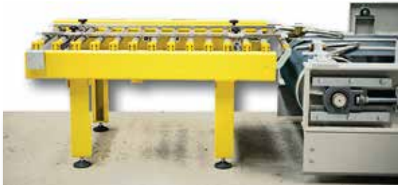
Motorlu ilave. Motorized roller conveyor.
