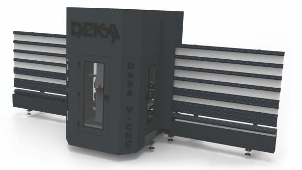
The FSR is a vertical machining center that combines multiple processes in a single machine, performing all tasks with speed and precision. The machine integrates vertical drilling, milling, polishing, and grinding operations, and can be used for any of the following processes on flat or shaped glass sheets. Its main feature is its versatility, allowing the machine to perform a wide variety of operations with speed and optimal precision.
