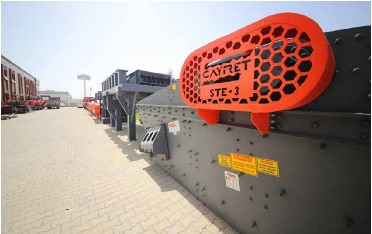
1600x5000 Yıkamalı Mobil Elek – 1600x5000 Mobile Washing Screen
