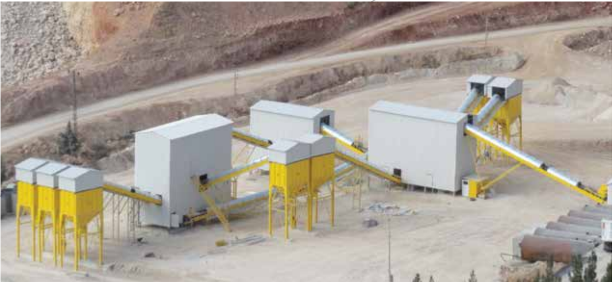
350 - 400 Ton Saat Kapasiteli Kırma Eleme Tesisi - Mardin 350 - 400 TPH Capacity Crushing & Screening Plant - Mardin
