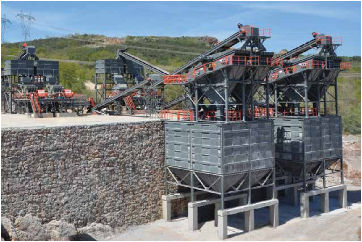
750-800 T/S Kapasiteli Kırma Eleme Tesisi - Sakarya 750-800 TPH Capacity Crushing Screening Plant - Sakarya
