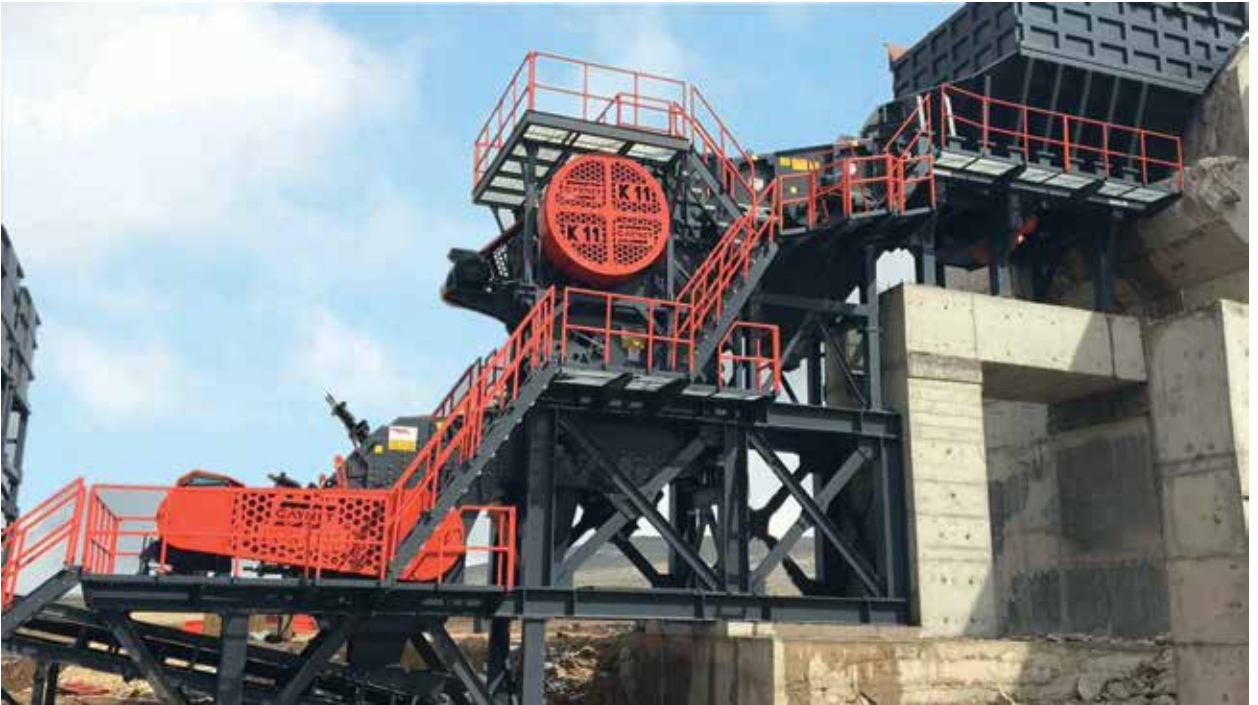
650 - 700 Ton Saat Kapasiteli Kırma Eleme Tesisi – Aksaray 650 - 700 TPH Capacity Crushing & Screening Plant Aksaray
