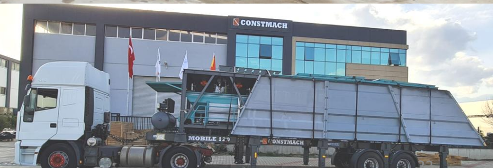
Transport position of 2nd chassis
