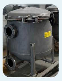
**Solid-Liquid Separation:** After the sugar beet juice is extracted, the remaining solid materials need to be separated. Pressure tube filter helps achieve this by filtering out the solids, resulting in clean sugar juice.
