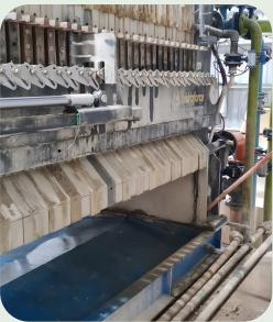
The dewatering of carbonation sludge is carried out in the HF-PF series filter press machines designed and manufactured by Hidroforce.
