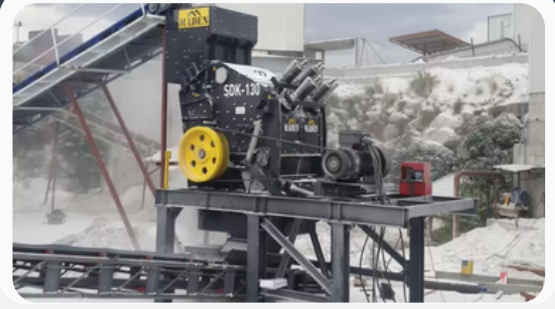
SECONDARY IMPACT CRUSHERS
