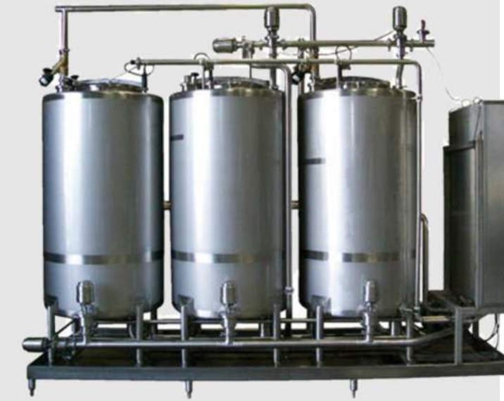
Cip cleaning unit
