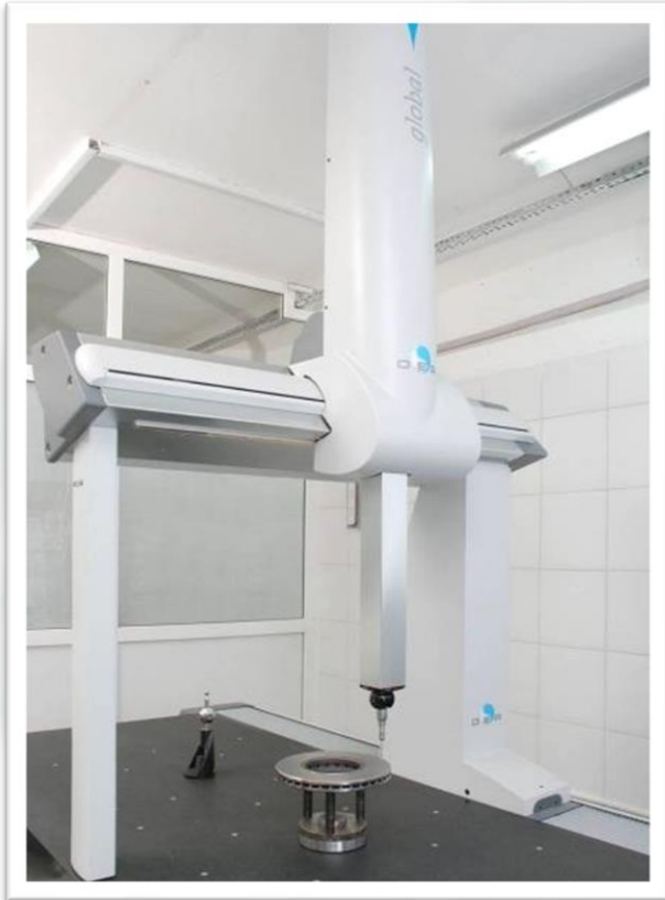
DEA 3D Measurement Machine 2000 x 1000 x 1000 mm
