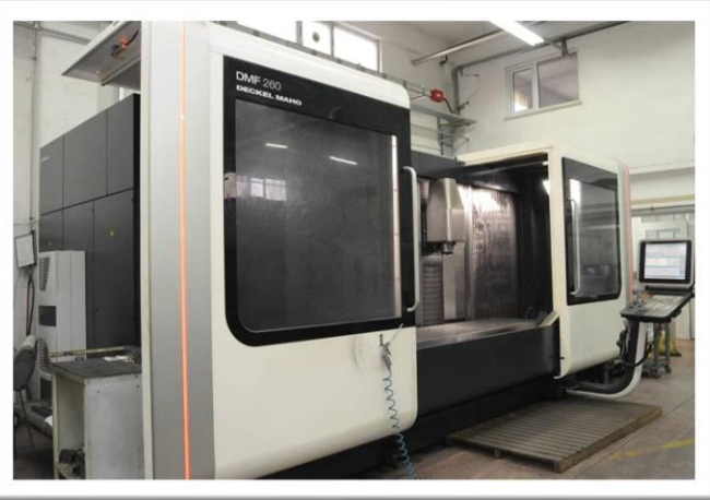
DMG 260 5 AXIS CNC Milling (X= 2,600 mm, Y = 700 mm, Z = 700 mm)
