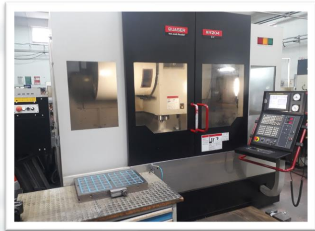
2 QUASER CNC Milling (X= 1,300 Y = 700 mm Z = 500 mm)
