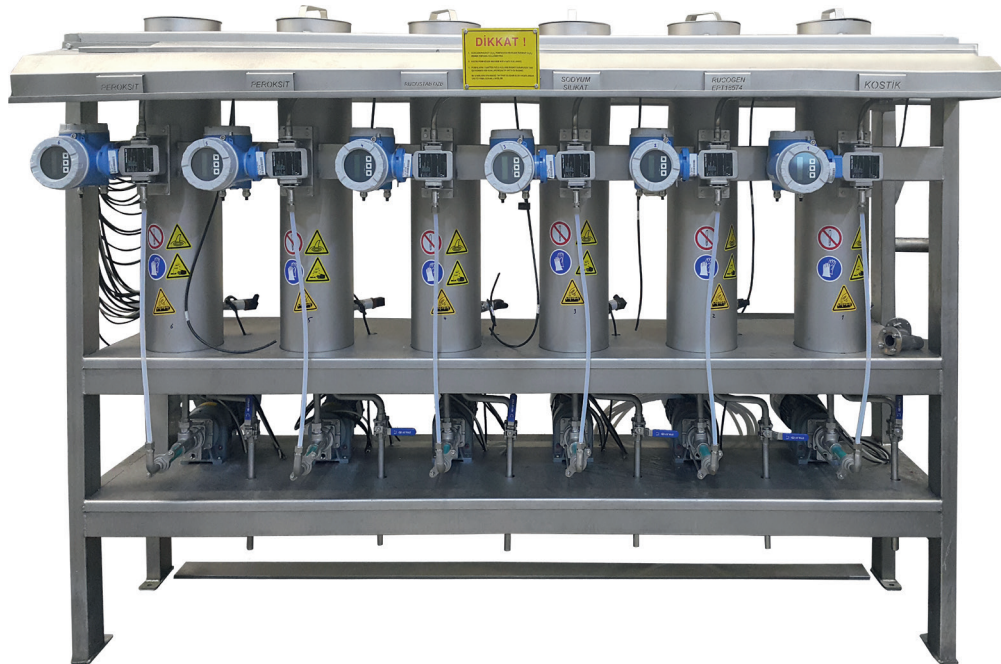
Kimyasal dozaj sistemi / Chemical dosing system
