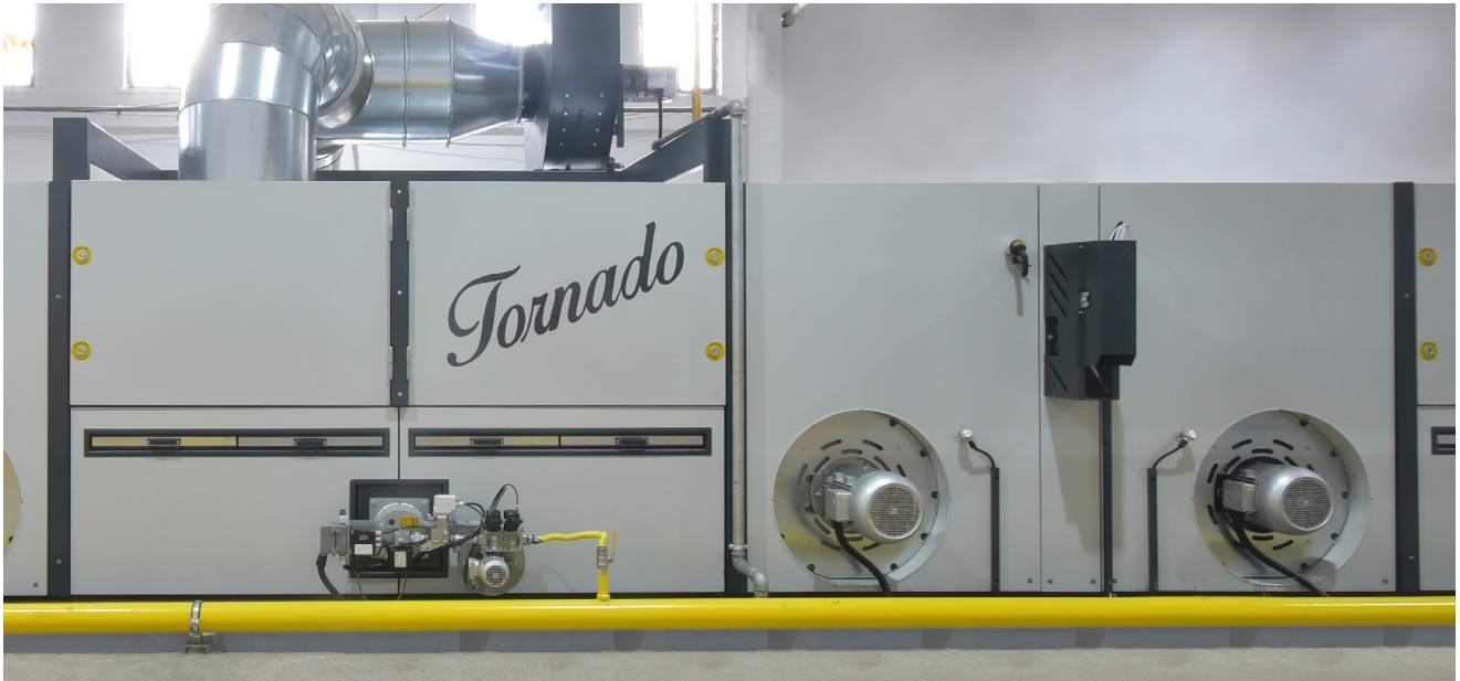
Tornado model chamber designed for higher air pressure and quantity specially woven heavy fabrics.
