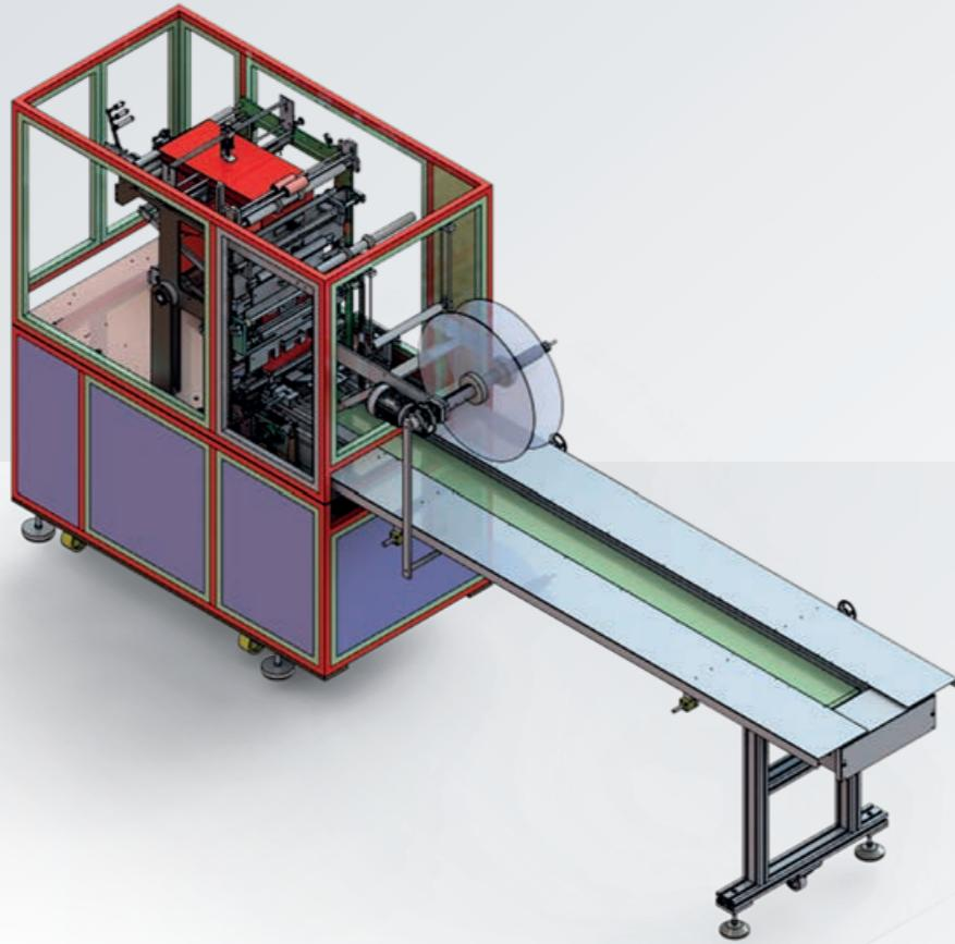
**NP-140** is a fully automatic overwrapping machine that is designed specially for the packaging of biscuit bundles, at medium to higher speeds.
