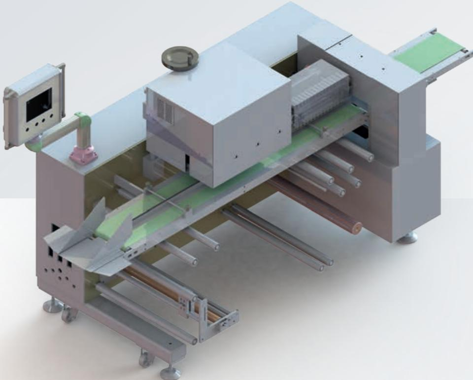
**NP-300** is all electronic, robust and simple to operate. It offers excellent solutions for all industry sectors, including automatic and manual supply lines. Flow wrapping which is also known as fin seal wrapping and horizontal bagging, is the process of wrapping a product in a clear or printed polypropylene film. The end result is a flexible package with a crimped top and bottom seal.
