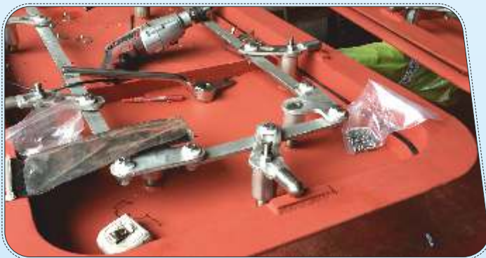
Watertight Steel Door
