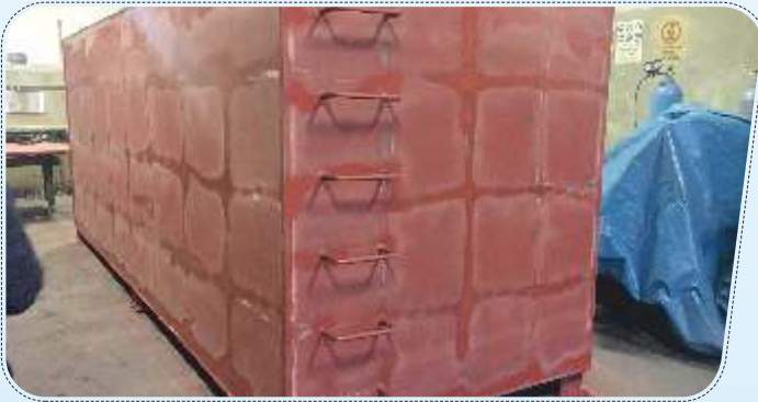
Main Fuel Tank
