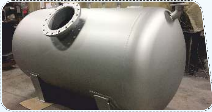
Pressurized Hot Water Tank (Painted)
