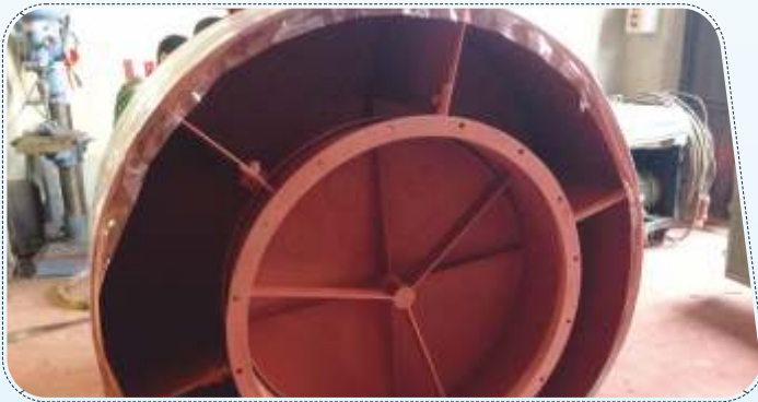
Painted Steel Ventilation Air Outlet Construction
