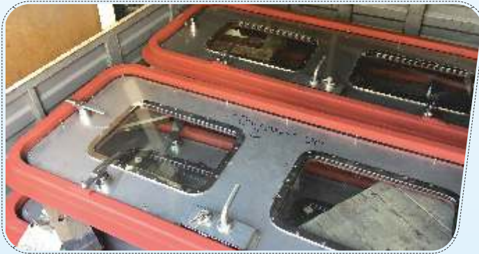
Steel Door with Glass and Stainless Steel Plate Inside
