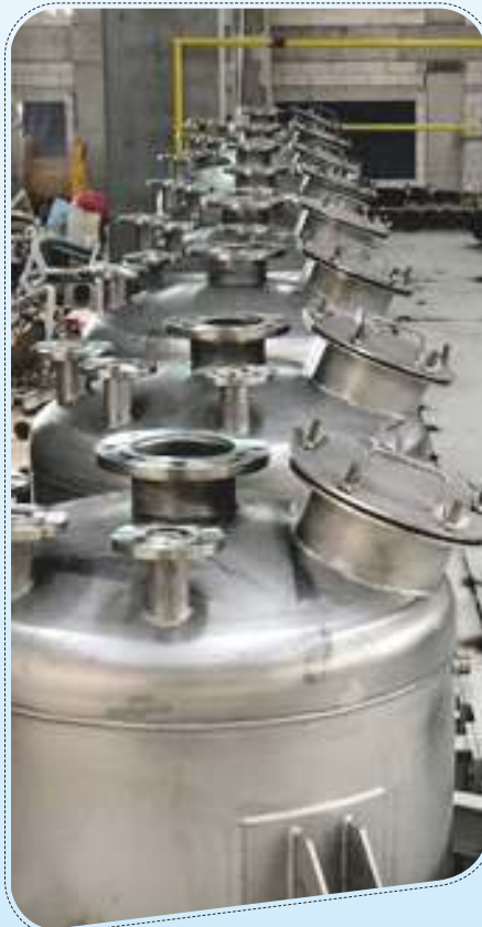
Stainless Steel Tank Farm Manufacture
