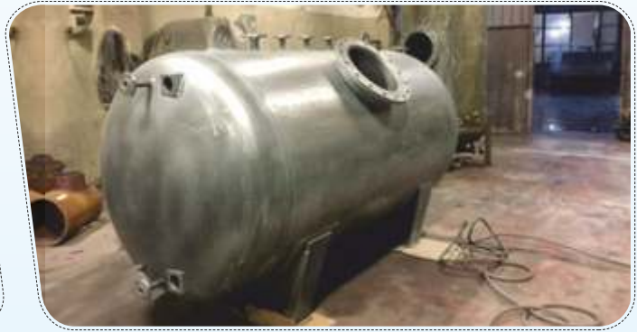
Pressurized Hot Water Tank
