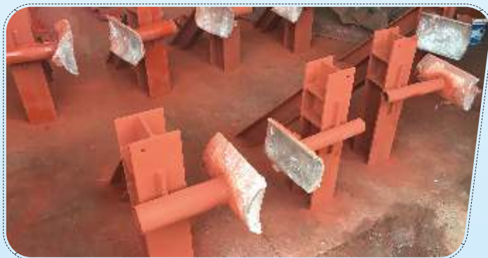
Tank Pipe Support (Painted)
