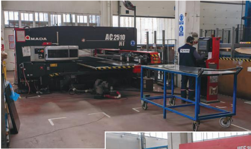
Raw Material Punching Process
