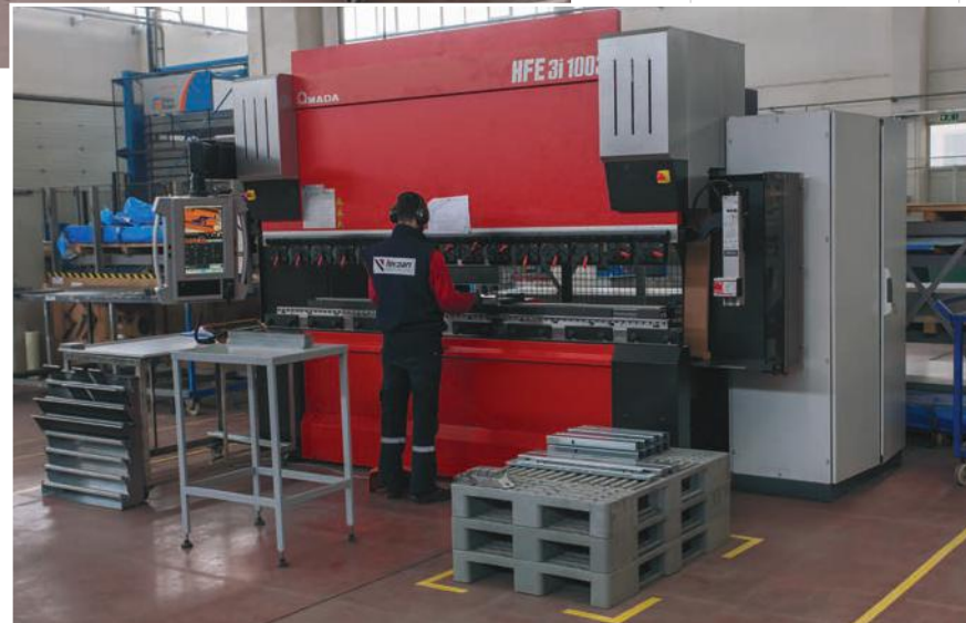
Raw Material Bending Process
