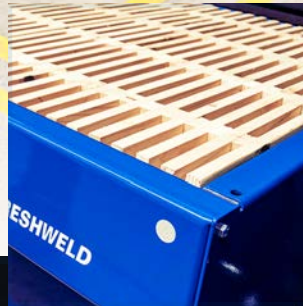
Modular Wooden Grid Your grinding products are protected from being scratched.
