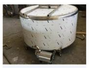
1000 Lt Vertical Type Milk Cooling Tank
