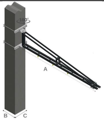
The SL-JC-COLUMN model mounted on the column is offered with 500 kg and 1000 kg carrying capacity options. Parameters A, B and C can be determined flexibly to best suit your needs and projects. The SL-JC-COLUMN model can be securely fixed to the column with the clamps located behind the joints. It is designed to offer a wide working area with the capacity of the compass to rotate up to 180 degrees.
