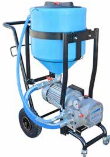
GIOTTO version on trolley with 50 litres gravity tank.
