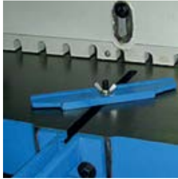
Açılı yaralanabilen ön dayamalar Front gauges with angle alignment
