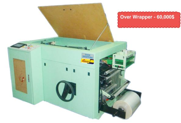
The ALEMIN OVER-WRAPPER wraps between 18 and 22 cigarette boxes per minute. Meets medium to high production requirements efficiently. Aleminsan over wrapper machines are able to wrap cartons flawlessly and smoothly. This machine is equipped with delta PLC controls to simplify operations.
