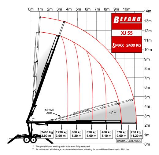
Equipping the device with a winch reduces the lifting capacity by 100 kg
