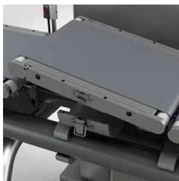
V-SHAPED BELTS for spherical and cylindrical products
