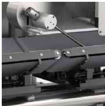
V-SHAPED BELTS for spherical and cylindrical products
