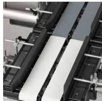
OPEN FLAT BELTS for thin packages
