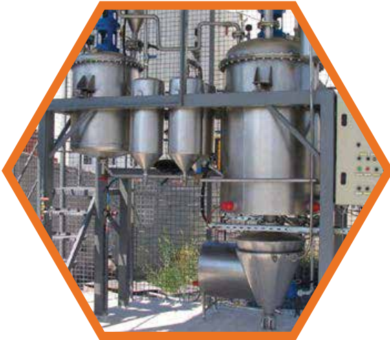
Biodizel Pilot Tesisi Biodiesel Pilot Plant
