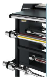
The drum is made of ST44 drawn steel pipe and all standard models are finished with surface grinding. On request the drum surface can also be plated with either chrome or Teflon. Inside the drum is an infrared heating element that operates without the use of any oil. The heat sensor is placed on the surface of the drum, this enables more accurate readings and provides better print results.
