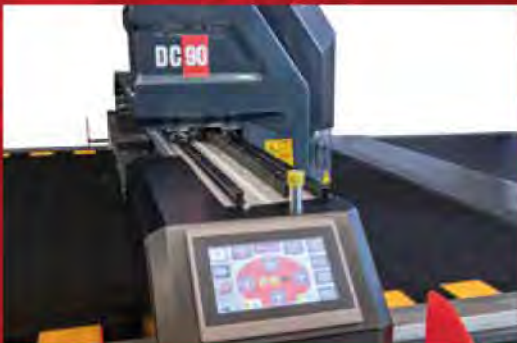
Özel seri kremayer dişli x ve y ekseni X and Y axis driven by Straight-Toothed Rack and Pinion
