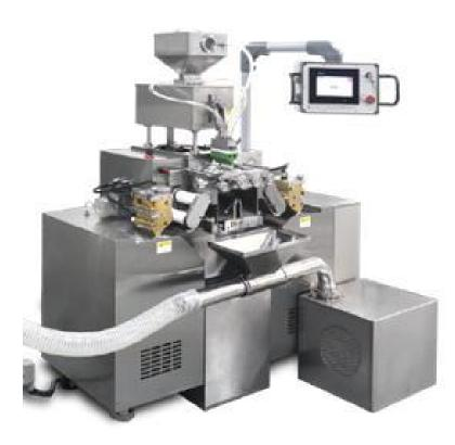
SINO-100 type mould-rolling soft capsule machine is a kind of new model according to SINO-100 model's performace & customer's requirement, with advanced design technician and information, and comform to GMP standard. With 220V power supply, it is mainly used for the soft capsule's developing in those small scale manufacturers or pharmaceutical research institute with the following characteristics:
