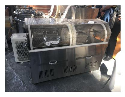
SINO-ZL100 type drying basket adopts frequency convertor to control, each joint can have positive or opposite running independently. One of or many of joints can be used at the same time. By controlling the rotation of the basket, pill can be kept in the current rotary drying, and also be pushed to the next to have the drying. Here are some advantages:
