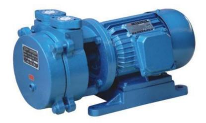
SN-1.5B type water-circulation vacuum pump is used to extract gas from the colloid melting vessel during the colloid solution preparation, so make the vessel be vacuum, then produce the colloid solution without bubbles. It's max air flow is 1.5 m³/minute, the limit vacuum is 700mmHg, the rotary speed is 2860RPM, the motor power is 4KW, and the water's consumption is 8-12L/minute.
