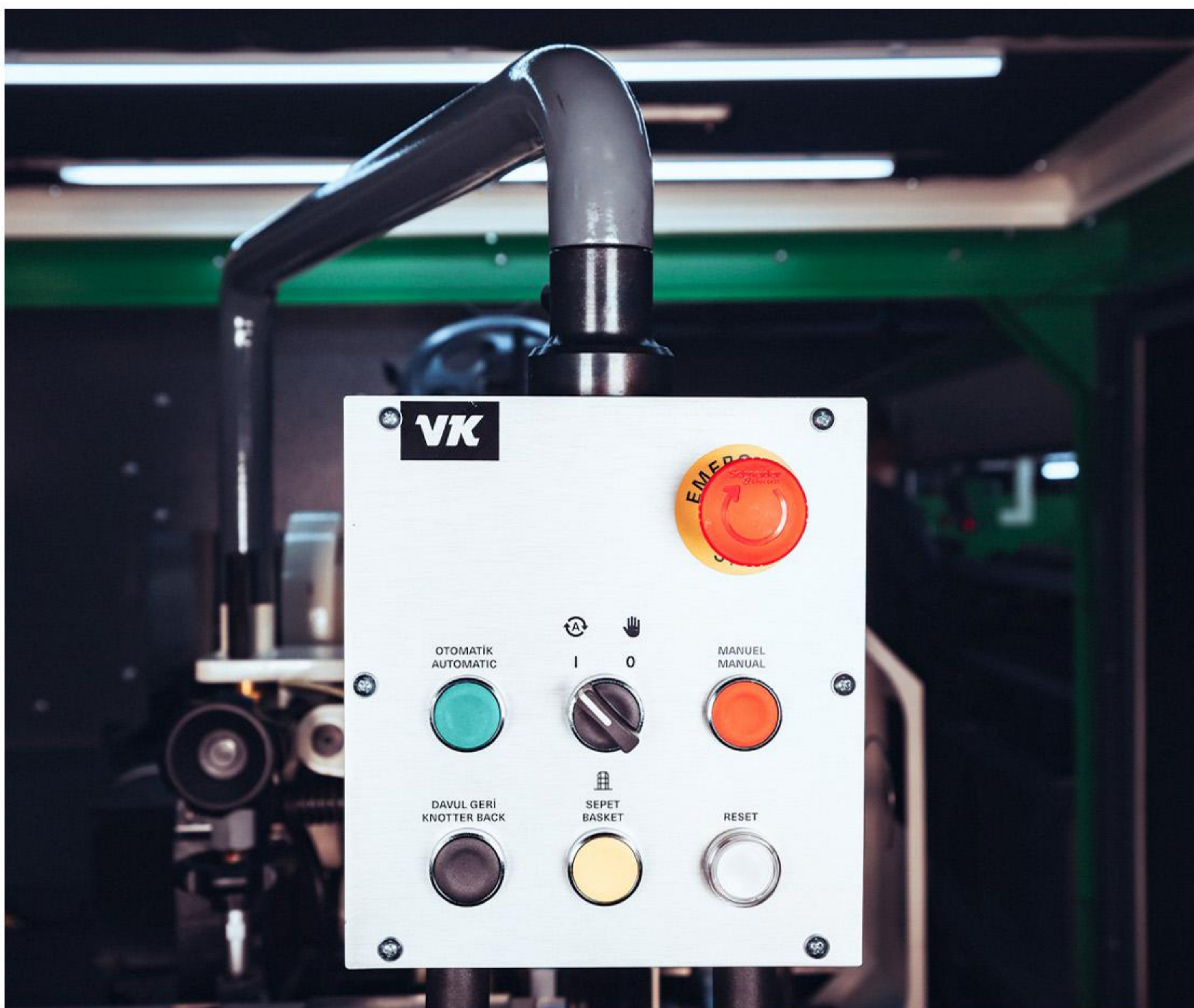
— Coiling Control Panel
