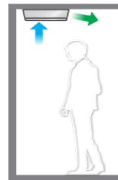
CEILING FIXING (only this configuration is possible for lifts and lifting equipment)
