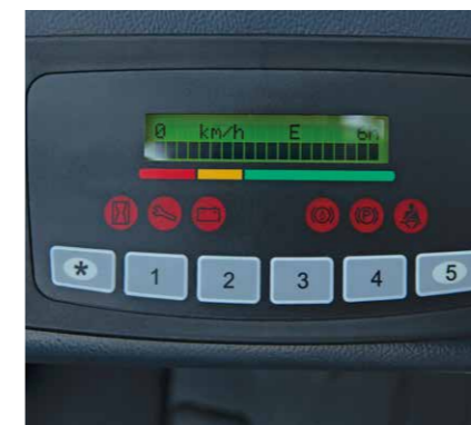
Zapi controller with multifunctional instrument panel
