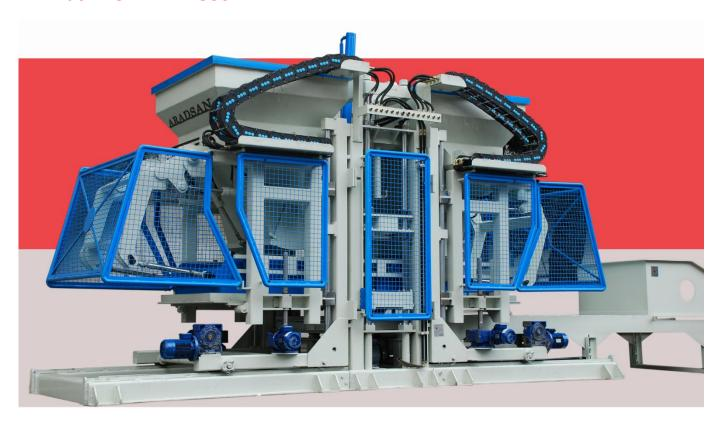
The system of TP.RN 2530 (special) can produce different types of concrete parts such as curbstones, paver and cement blocks.
