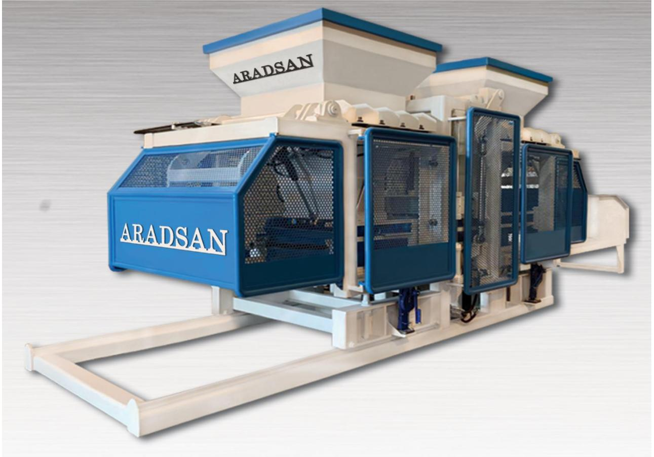
Automatic Concrete Block Machine TP.RN1518 II Double Packet can produce different kinds of concrete parts (curbstone, block, pavers ,interlocking bricks , flower box). It is presented in two types (single packet and double packet). The production capacity in the single packet system is %10 more than double packet , and the other difference is in the dual-color production capabilities of the double packet system.
