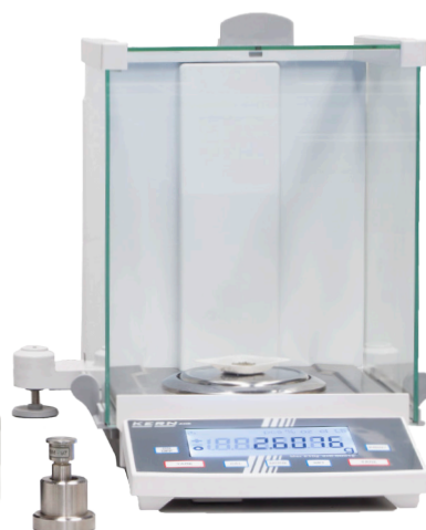
AUTOBLAINE PREMIUM connected to analytical balance
