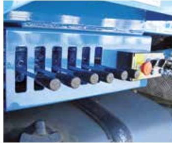
MANUAL CONTROL DIRECTLY ON THE MAIN VALVE
