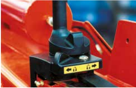
INTERLOCK SYSTEM SAFE CRANE OPERATION
