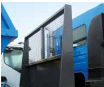
PROTECTIVE WALL BETWEEN CAB AND CONTAINER
