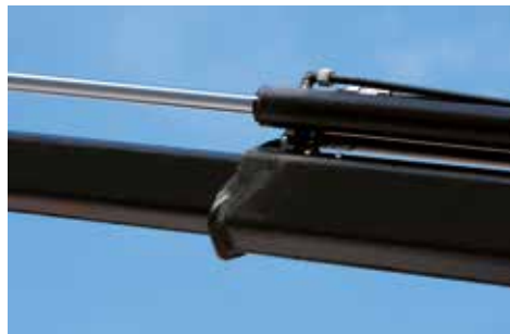
INTERNAL OIL FEEDS MAXIMUM PROTECTION THANKS TO COMPACT DESIGN
