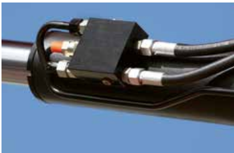
HYDRAULIC OVERLOAD PROTECTION SAFE CRANE OPERATION
