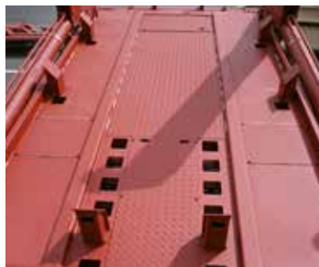
ADJUSTABLE CONTAINER STOPS – LENGTHWISE / SIDEWAYS
