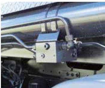
CHECK VALVES ON EACH HYDRAULIC CYLINDER
