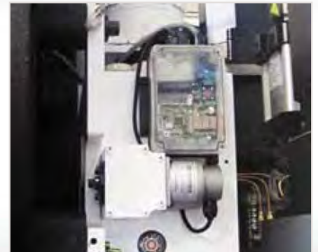
■ Absolute Encoder ATC System < NXV1680B is exclusive >
