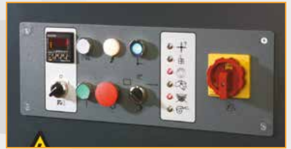
Control panel with optic indicators of operation anomalies
