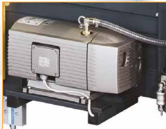
Vacuum pump for box keeping
