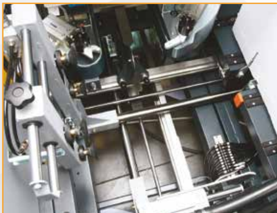
Pneumatic cylinders for box moving and box squaring
