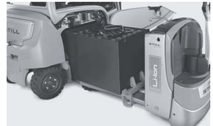
Battery changing with electric pallet truck
