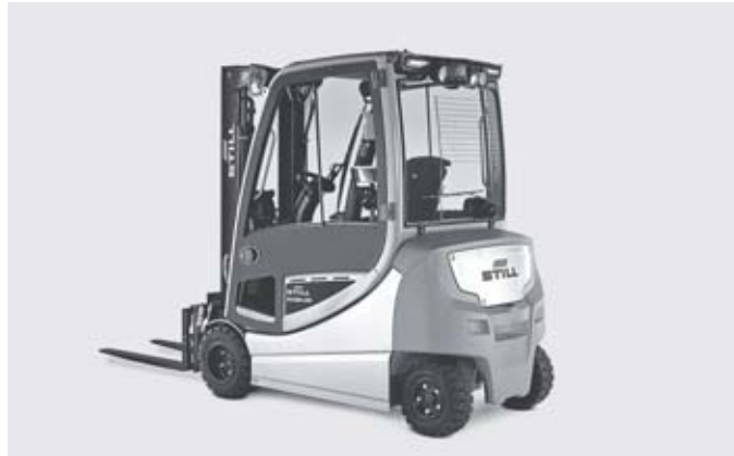
Four-wheel version with fully enclosed driver's cabin for outdoor use
