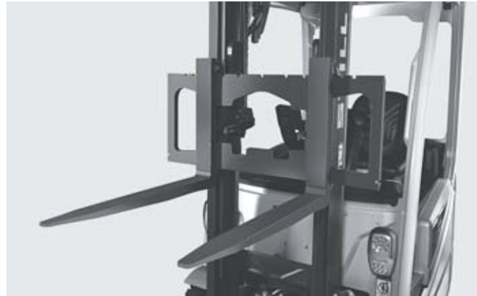
Optimal view of fork tips when loading HGVs
