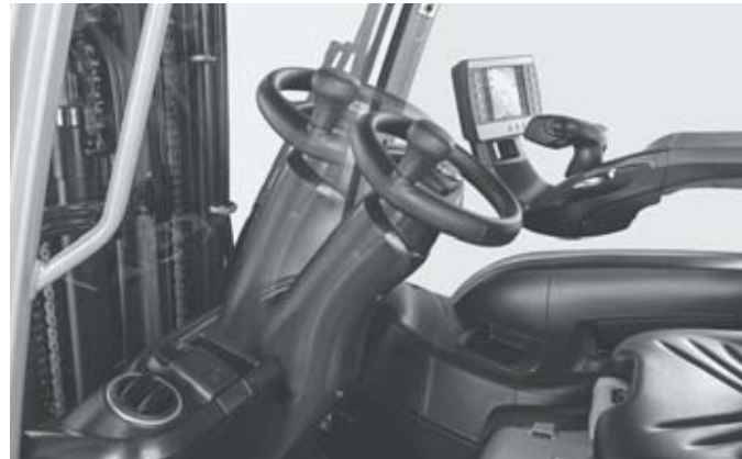
Driver's seat steering column adjustment up/down
