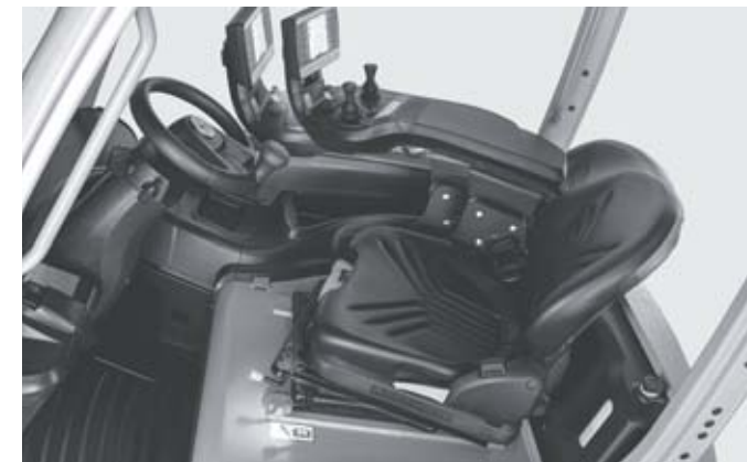
Swivel seat for comfortable reversing
